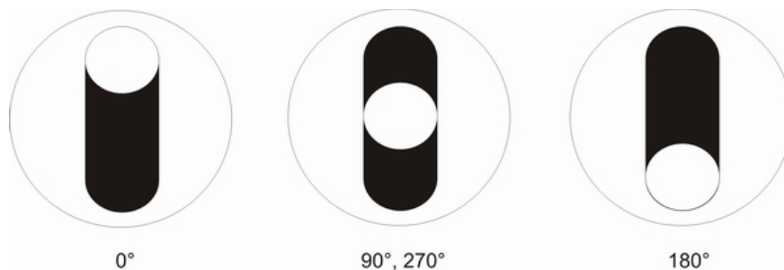
End views of Rotor turning in Stator as the Rotor completes one revolution
